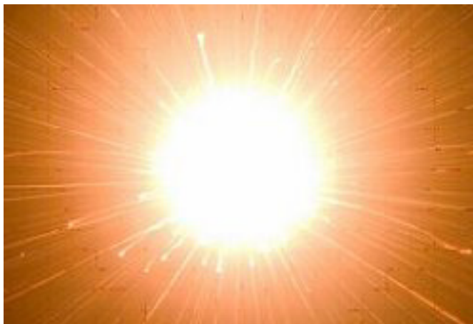
A simulated meteoroid explodes on impact at the NASA/Ames Vertical Gun Range. This is a genuine photo showing the spray of secondary particles
