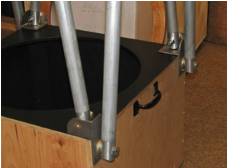
Truss brackets machined by Tom Conlin for club's 18" scope
